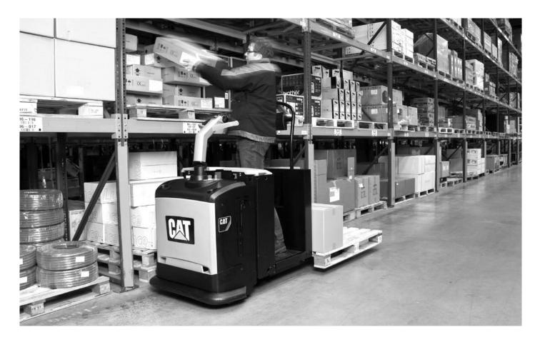
The NO20NT low-level order picker is designed for fast and safe handling of orders from the picking face to despatch.
